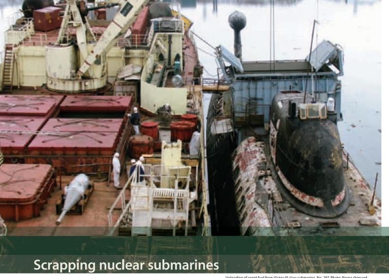
$Unloading\ of\ spent\ fuel\ from\ Victor-III\ class\ submarine, No.\ 297.\ Photo:\ Nerpa\ shipyard.$
