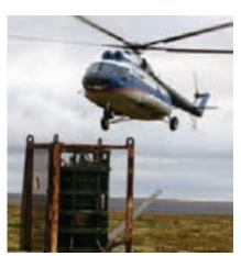
At inaccessible locations, the RTGs must be shipped out using helicopters. Photo: County Governor of Finnmark.
