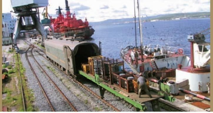
$Reloading\ RTGs\ from\ ships\ onto\ special\ trains\ at\ RTP\ Atomflot\ in\ Murmansk.\ Photo:\ County\ Governor\ of\ Finnmark\ at\ County\ Governor\ at\$
