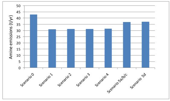
Figure 10-4: Estimated amine emissions from the carbon capture plant
