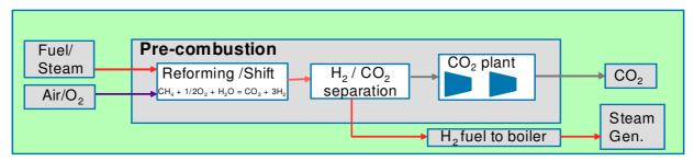
Figure 3-6 Pre-combustion steam generation
