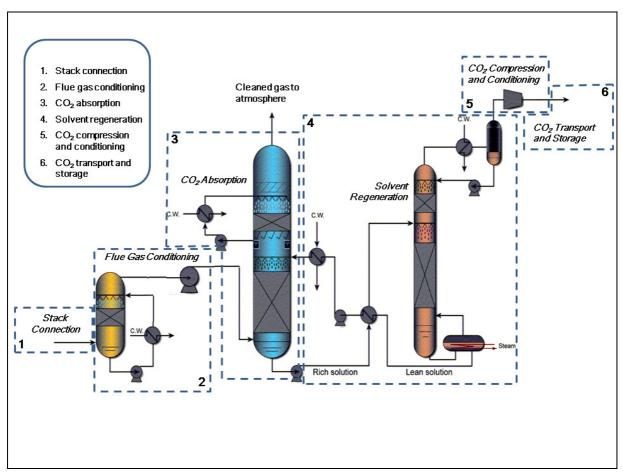
Figure 3-3 Typical amine based carbon capture and compression plant (Source: SINTEF)
