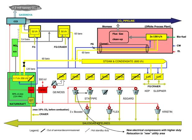
Figure 6-10 Schematic overview of scenario 5b
