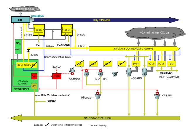
Figure 6-7 Schematic overview of scenario 4
