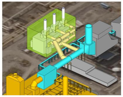
Figure 6-20 Layout exhaust stack and high pressure boilers system scenario 5d
