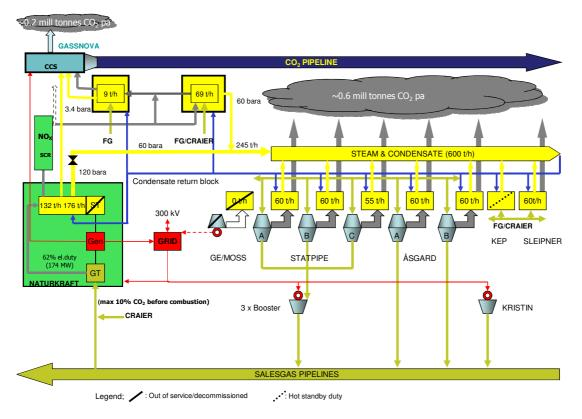
Figure 6-6 Schematic overview of scenario 3
