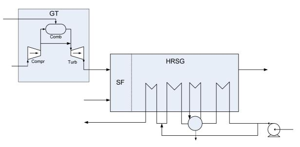
Figure 10-1 Gas turbine and heat recovery unit model
