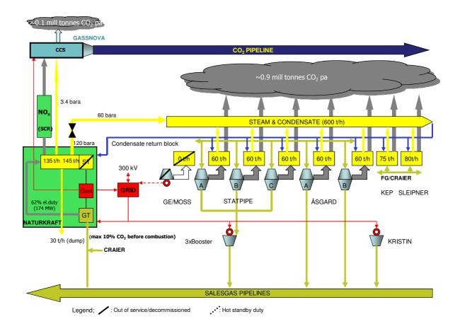
Figure 6-5 Schematic overview of scenario 2
