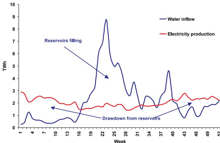
**Figure 2.1** Variations in water inflow and electricity output during a year
