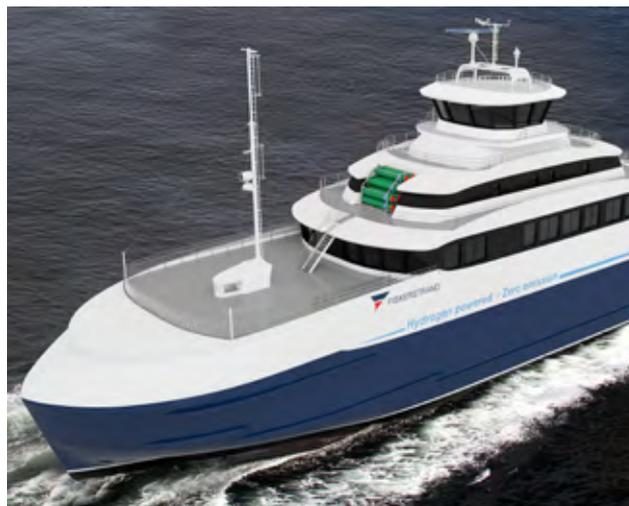
Concept sketch of the hydrogen ferry, powered by fuel cells and batteries
