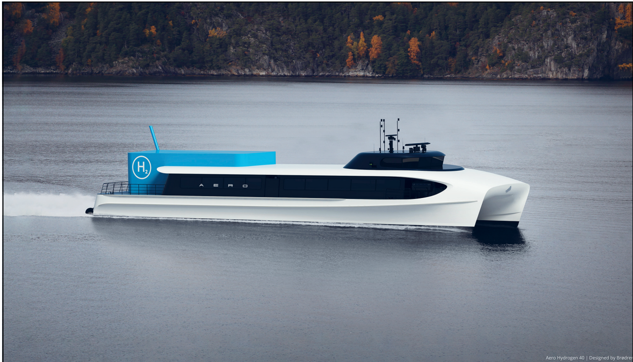
Figure 3.19 Zero-emission high-speed vessels of the future may look like this. The Aero Hydrogen 40 concept was developed by Brødrene Aa in collaboration with Westcon Power and Automation, Boreal and Ocean Hyway Cluster. The 277-passenger vessel will be battery- and hydrogen-powered and reach 34 knots, with an output of 2 600 kW.
