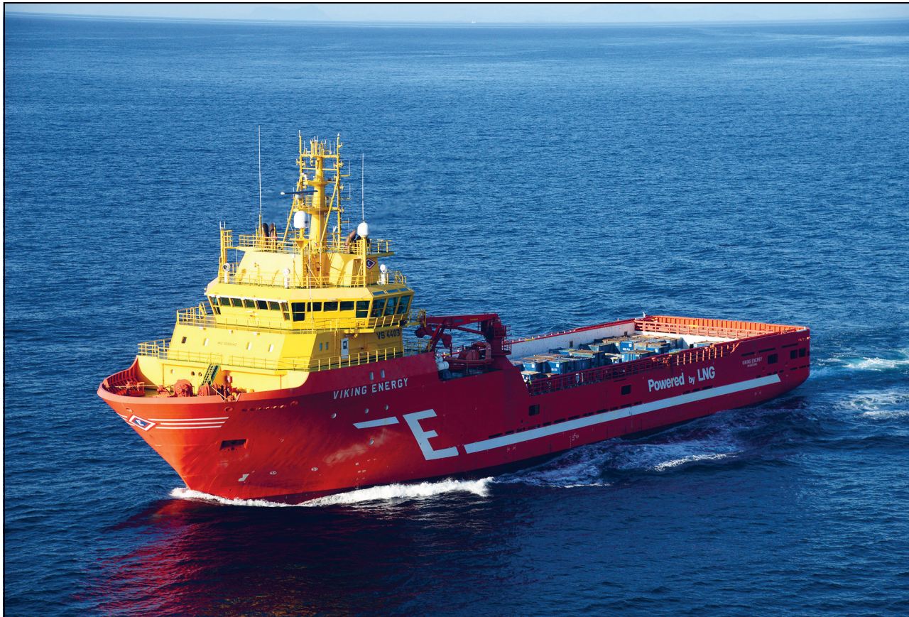
Figure 3.20 The offshore supply vessel Viking Energy is being retrofitted to use ammonia as fuel from 2024.
