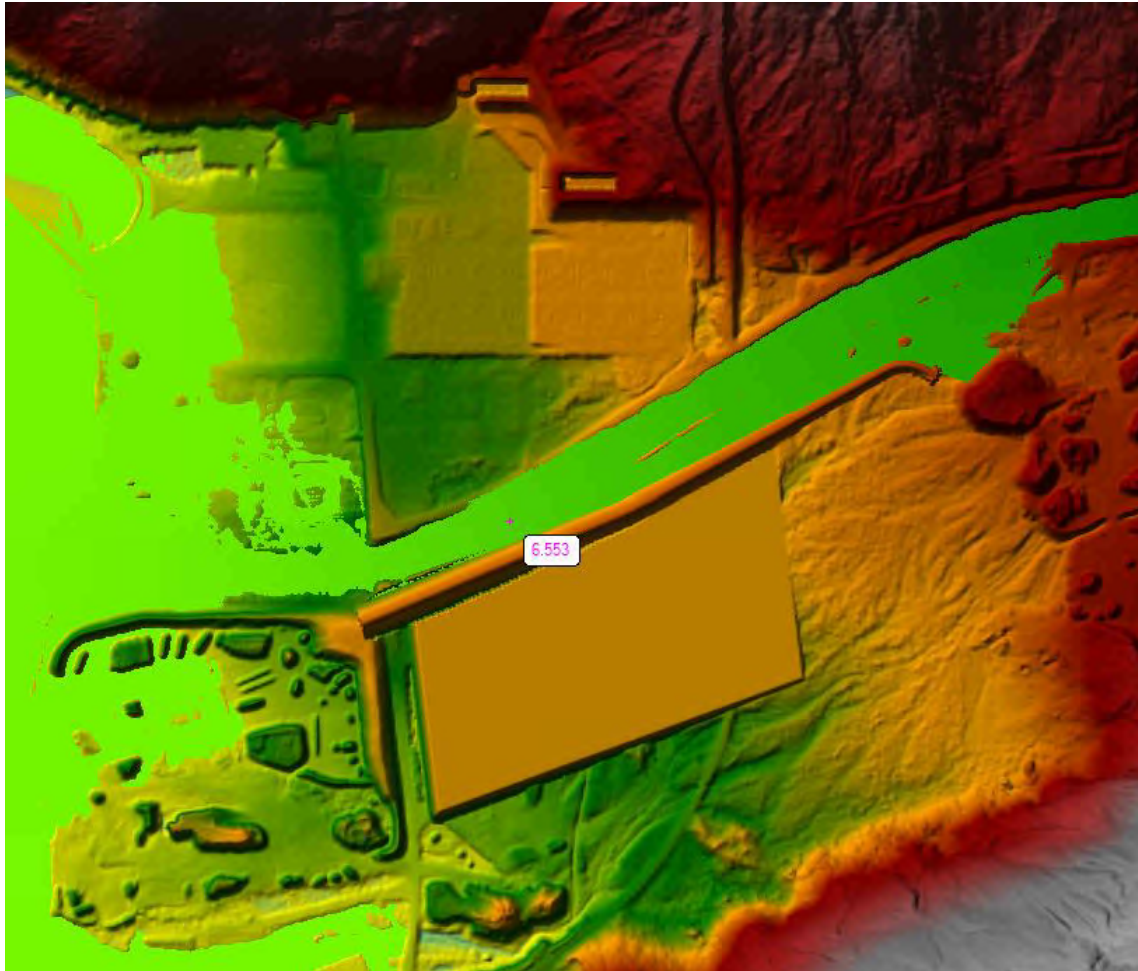
Figure 50 Analysis of "simulated levees on both sides to compare with 1D model. Compared with results in Figure 21 (cross section 6), calculated water surface is similar for Q=185\text{m}^3/\text{s} . Analysing simulated water surface levels at cross section 6. Manning n \sim 0,06 - 0.066 gives similar results as the 1D model. Analysis without false levees, see Figure 51 and Figure 52
