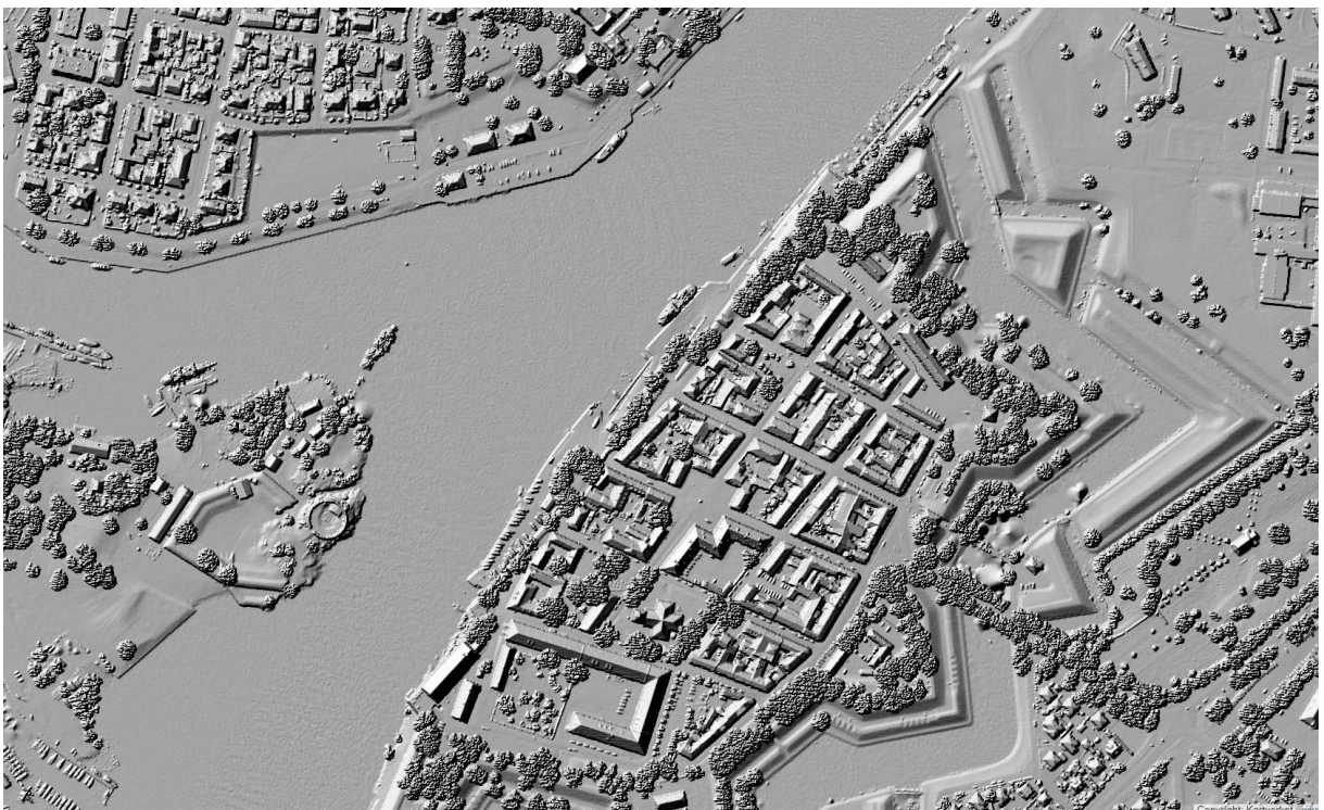
Figure 1.1 A surface model showing elevation data based on detailed laser measurements from an aircraft
