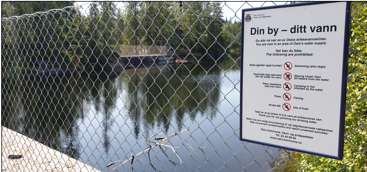
Figure 4.10 Signage and fencing of drinking water sources is an important and sound measure to avoid water contamination.
